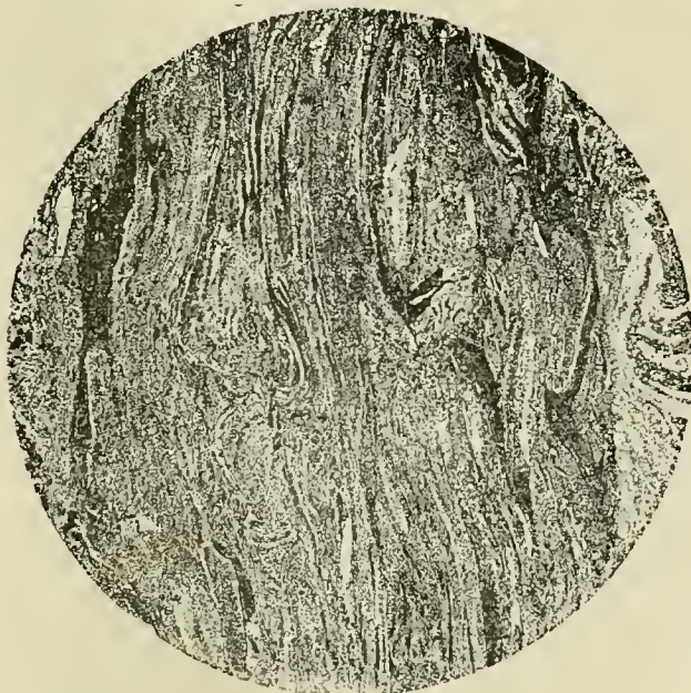
Section of Wrought-Iron Axle.
